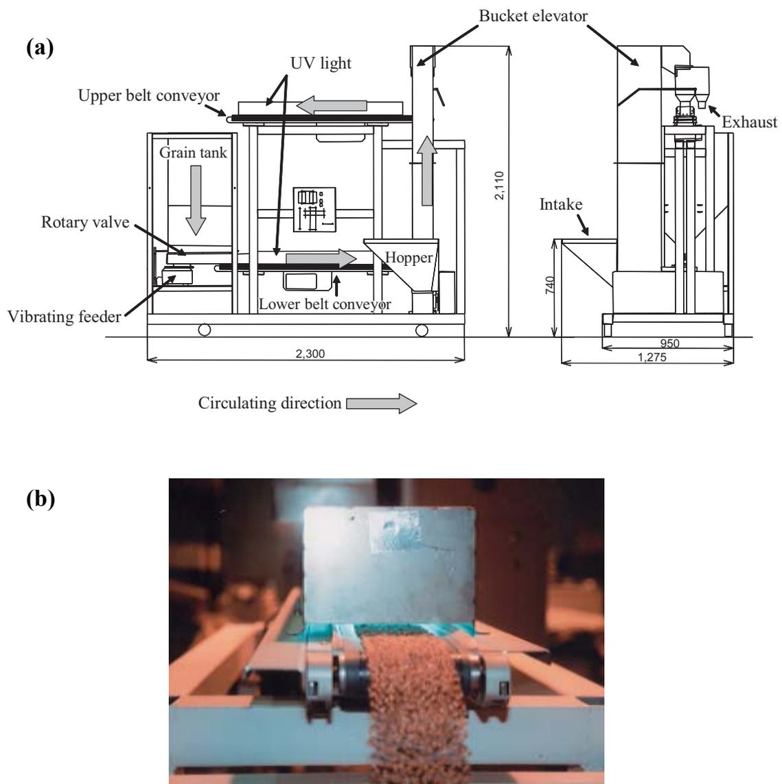
**Fig. 1. Schematic diagram of recirculating grain sterilization equipment using ultraviolet irradiation**
