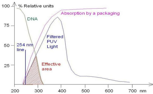
On the left is the effective sterilization emission through a UV-semi-transparent packaging material (on the right):
