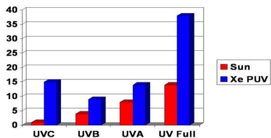
The Solar UV has significantly less UV because the effective visible temperature of the Sun is also far less: 5780°K.
