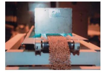
Fig. 1. Schematic diagram of recirculating grain sterilization equipment using ultraviolet irradiation
